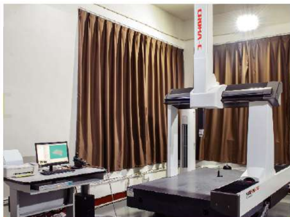
瑞典海克斯康三坐标测量仪 Trilinear coordinates measuring instrument from Sweden Hexagon
