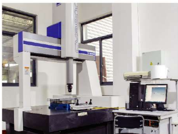
德国蔡司三坐标测量仪 Trilinear coordinates measuring instrument from German Zeiss
