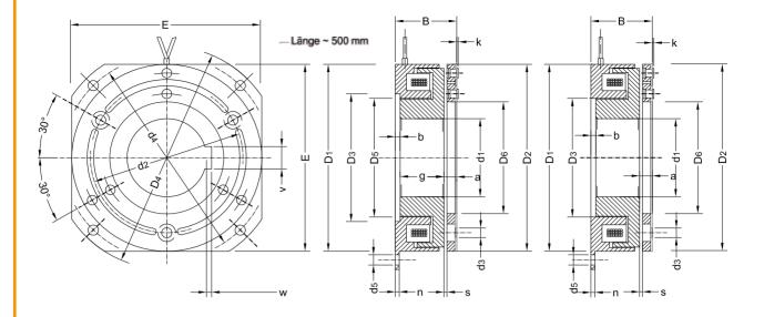
**Dimensions: Single disc clutches**Dry run DC 24V (different current on request)
