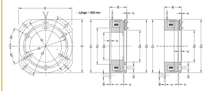
**Dimensions: Single disc brakes**Dry run DC 24V (different current on request)
